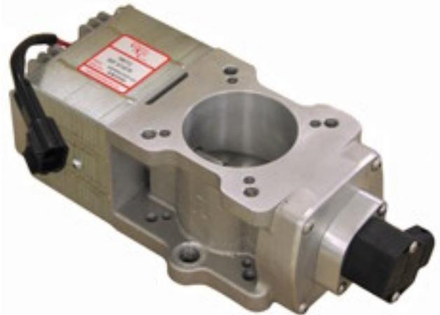
The ATB SERIES design uses steel, precision grade radial ball bearings to provide low friction support to the throttle shaft. Therefore, no maintenance is necessary. The results are a rapid, proportional response to actuator positional changes and outstanding reliability consistent with GAC expectations.
